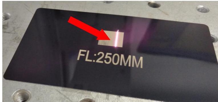
Less than the correct FL (比正确焦距短)
